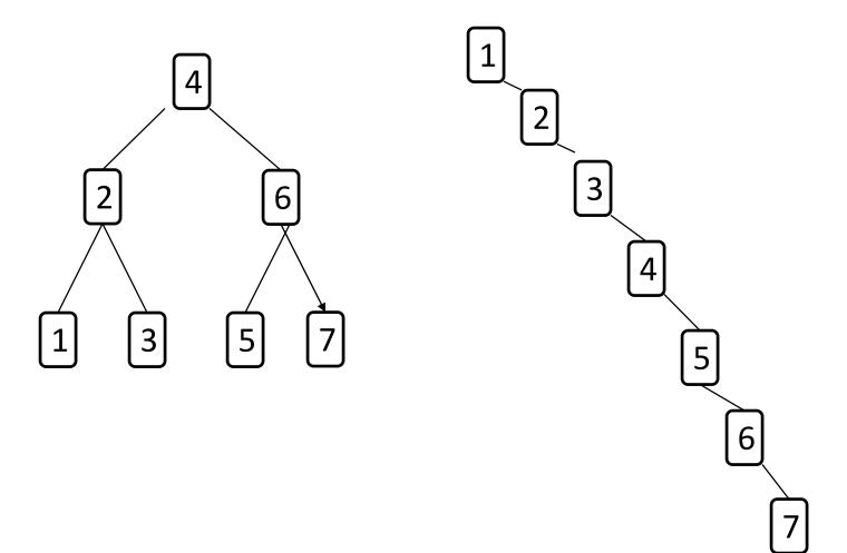
This tree is *balanced*. All of the nodes at a given depth have the same numbers of nodes in their left and right subtrees. The find(), add() and remove() algorithms for balanced binary trees all have O(log(n)) *running time*.
