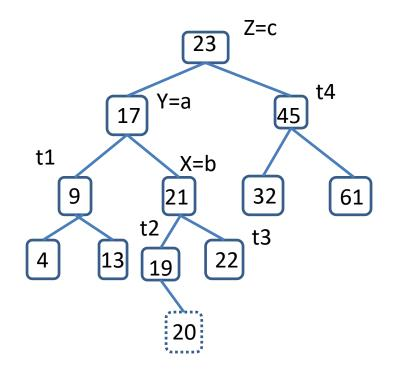
Once we have Z, Y, and X identified we can label a, b and c as those same nodes in increasing order, and we identify t1 through t4 as the children of a, b, and c. We can now rebuild the tree:
