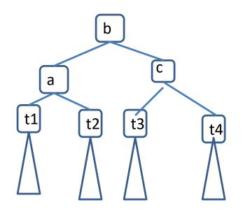
Furthermore, t1 and t2 have the same relation to a as before, all of the values in t3 are greater than the value of b and less than the value of c, and t4 remains the right child of c. This means that the new tree is a Binary Search tree that satisfies the AVL property. Case 2: Y is Z's right child, X is Y's right child. This is symmetric to case 1
